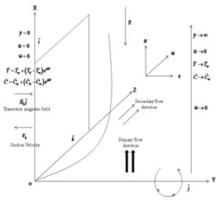
Figure 1. Flow configuration.
