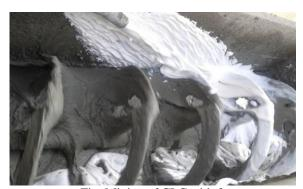
Fig. Mixing of CLC with foam
