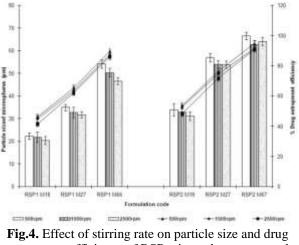
entrapment efficiency of RSP microspheres prepared using PLGA of varying molecular weights.
