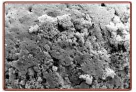
**Fig.10.** SEM photomicrograph of degraded RSP-PLGA microspheres prepared using PLGA (75:25) after 28 days.
