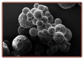
Fig.9. SEM photomicrograph of RSP<sub>2</sub>M27 microspheres.
