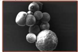
Fig.6. SEM photomicrograph of RSP<sub>1</sub>M66 microspheres.
