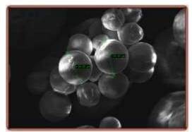
Fig.7. SEM photomicrograph of RSP<sub>1</sub>M27 microspheres.
