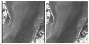
Fig 6: Lost column modification algorithm for coastal areas, original image (left) and after modification (right)
