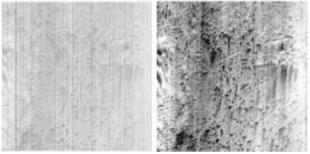
Fig 3: Lebanon desert image in band 1 before de-striping (left) and after de-striping (right)
