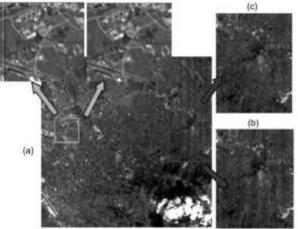
Fig 5: (a) Original image taken by CHRIS sensor (b) Area affected by residual stripes close to a columns of clouds (c) The same area mitigated by the use of bright pixel masking
