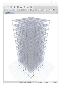
Figure7. Building without Shear wall
