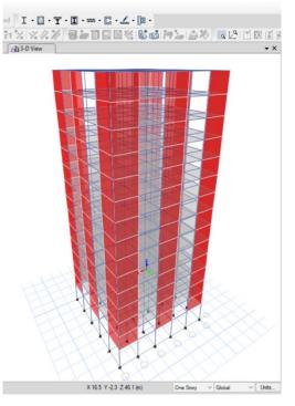
Figure 6. Building with Shear wall
