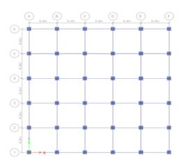
Figure 2. Plan of Building Without the Shear wall
