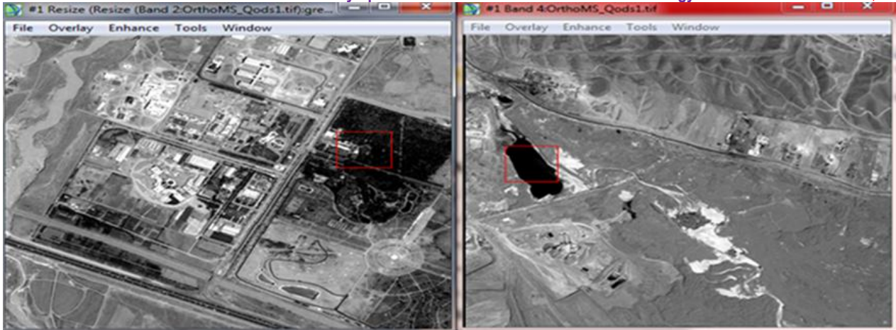
Fig(1). Separating image into green and near infrared bands: the right image represents a body of water in the near infrared band and the left one shows trees in the red band.
