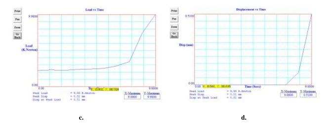
Fig .7. Tesile test graph for butt weld at 870 rpm. (a) Load vs Displacment, (b) Stress vs Strain, (c) Load vs Time (d) Displacment vs Time.
