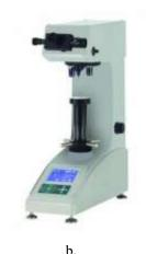
Fig .3. (a) Vicker's hardness test specimen, (b) Vickers hardness tester [16].
