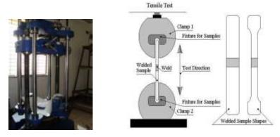
Fig. 4. (a) Tensile Machine, (b) Schematic diagram of tensile specimen and Fixture.
