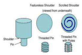
Fig.1. Schematic drawing of the FSSW tool.
