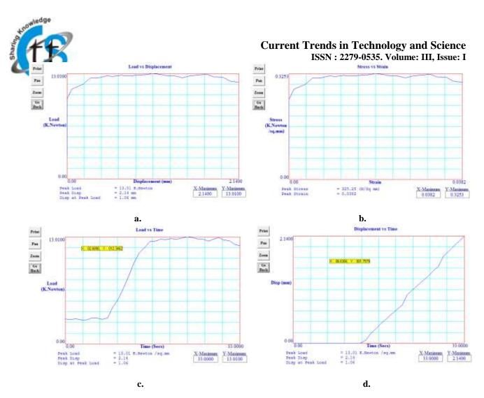
Fig .8. Tesile test graph for butt weld at 870 rpm. (a) Load vs Displacment, (b) Stress vs Strain, (c) Load vs Time (d) Displacment vs Time.
