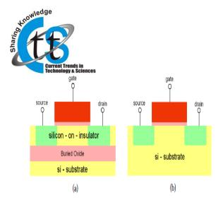
Fig.2. MOSFET structure of: (a) SOI b) conventional bulk
