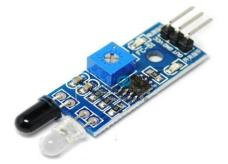
Figure 2: IR Sensor HDLC-4260
