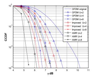
Figure 4 PAPR comparison for original SLM, Improved SLM and AMR SLM
