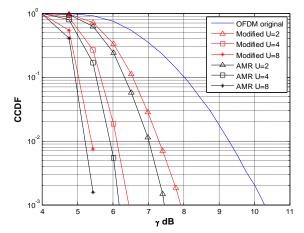
Figure 3 PAPR comparison for original SLM, modified SLM and AMR SLM
