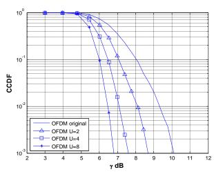
Figure 1 PAPR comparison for classical SLM
