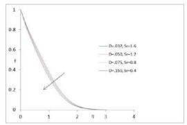
Figure 4 Velocity Profile for different values of D, Sr for v = 0.5, Da =0.5 and M =0.3
