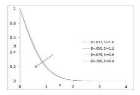
**Fig 5** Temperature Profile for different values of D, Sr for v = 0.5, Da =0.5 and M =0.3
