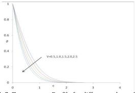
Fig2. Temperature Profile for different values of v for Sr = 2.0, D = 0.03,Da = 0.5 and M = 0.3
