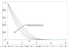
**Figure1** Velocity Profile for different values of v for Sr = 2.0, D = 0.03, Da = 0.5 and M = 0.3
