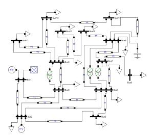
Fig-1: IEEE-14 bus network without DG connection
