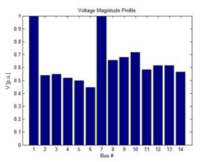
Fig-4: Voltage profile without DG connection
