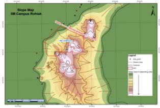
Figure 5: Slope Map showing streamlines and sink points
