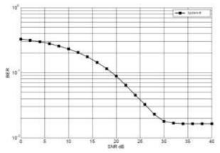
Fig. 3 Performance of matched filter based NML detector (system B)
