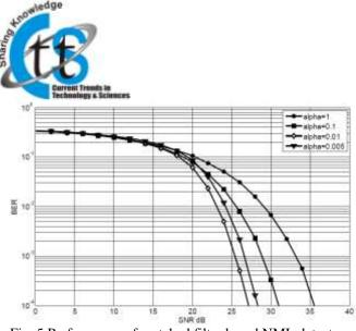
Fig. 5 Performance of matched filter based NML detector (System D)
