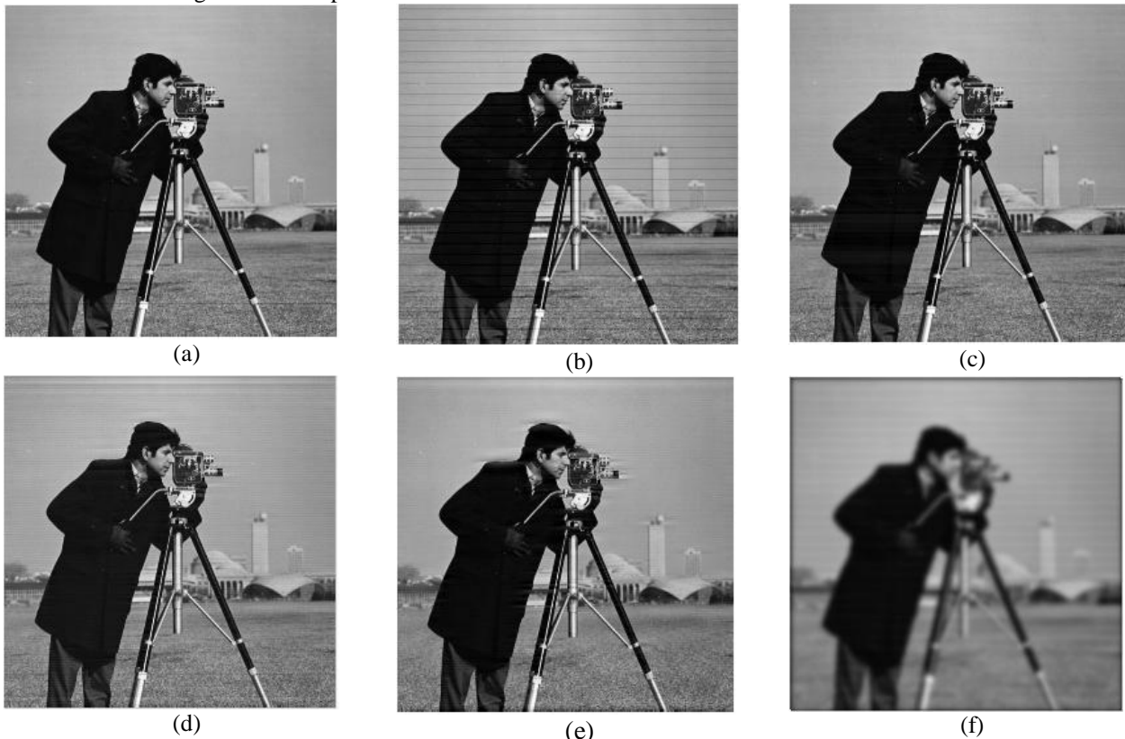
Fig. 6. A) original image, b) simulated image c) corrected image using wavelet-based filter, d) corrected image using order one Butterworth notch filter e) corrected image using spatial domain filter, F) corrected image using Gaussian low-pass filter with a standard deviation of 2.
