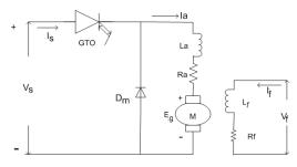
Fig.2 Chopper fed SEDC motor
