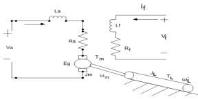
Fig.1 Dynamic model of separately excited DC
