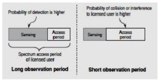
Fig 7: Trade off between spectrum sensing time and user throughput [25]
