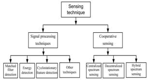
Fig 8: Various spectrum sensing techniques.
