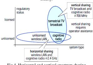
Fig.4. Horizontal and vertical spectrum sharing techniques
