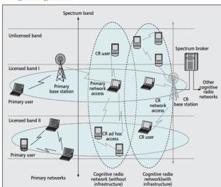
Fig. 1. Cognitive Radio Network Architecture
