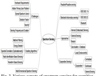
Fig. 3. Various aspects of spectrum sensing for cognitive radio.
