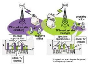
Fig.6. Cognitive radio in the TV band: At different locations, the cognitive radio devices detect different frequency channels as free and interpret them as opportunities for their own communication. This example for vertical spectrum sharing is discussed at IEEE 802.22<sup>™</sup> standardisation.
