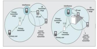
Fig. 2. : Some issues faced during spectrum management Transmitter detection problem: a) receiver uncertainty; b) shadowing uncertainty.
